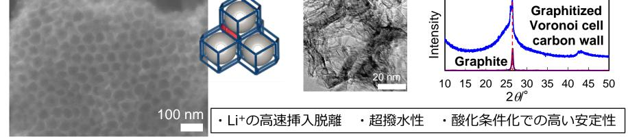
Figure (from left to right). Field emission scanning electron microscope, transmission electron microscope, and X-ray diffraction pattern of carbon nanowall assembly. Schematic diagram of regularly self-assembled polystyrene particles used as a template (neighboring 4 particles are shown here) and edges of rhombic dodecahedrons as the Voronoi cell are also shown. The cell walls are situated between the polystyrene particles, and one of them is shown in red.
